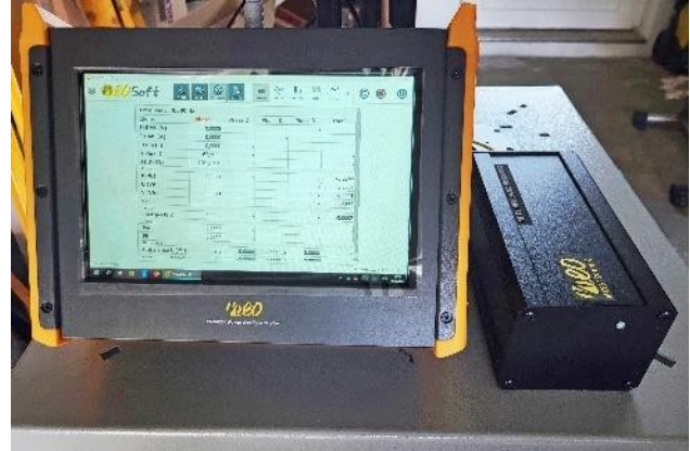
Figure 14 Prototypes of a commercial measuring device for a combined PQ and grid impedance measurement
