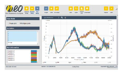
Time- and frequency dependent characterization of the grid impedance
