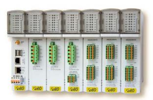
PQM-100 is based on modular architecture, allowing combination of one CPU module and up to 6 selected input modules into one device. The input modules are providing input signal isolation, filtering and A/D conversion. The CPU module is equipped with FPGA real-time controller for the calculation of all parameters and to provide all interfaces and data storage.
