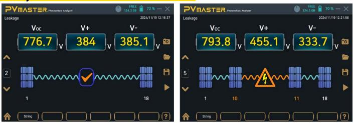
The safety measurement is used to determine whether leakage currents occur on the string. This measurement provides protection for both the measuring device and the technician. The benefit of this measurement is that the location of the fault is displayed as well.
