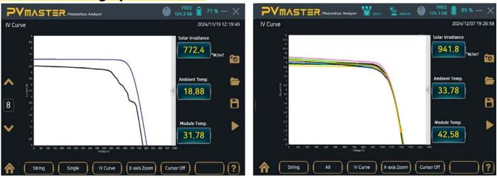
The measured IV (**up to 2200 data points**) curve is compared with the reference curve. The differences between the two indicate different errors. A total of 1-20 strings are measured per measurement. The analysis can then be carried out using the various software tools. This measurement can be carried out on **any type of module**, such as **N-type**, **P-type** and even **high-capacitance modules** with **inrush currents up to >200A**.
