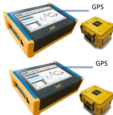
Example damping analysis of PLC transmission by measuring grid impedance at two points (Smart Meter and transformer station) with high precision time synchronisation
