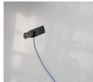
Thermal couple on the back of photovoltaic module
